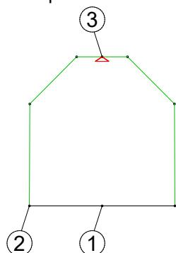
Verification point 2 is decisive for the chords. To be on the safe side, it is assumed that the entire cross-section is located in the heat-affected-zone (HAZ).
