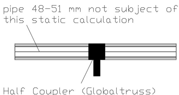
The pipe 48-51 mm is not part of this static calculation and must be verified separately!
