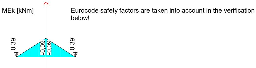
Verifications at point 1 - Verification horizontal pipe: (including safety factor 1,5 according to Eurocode)
