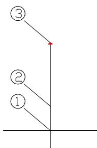
The decisive factor for verifying the horizontal tube is point 1. To be on the safe side, it is assumed that the entire cross-section is located in the heat-affected-zone (HAZ).
