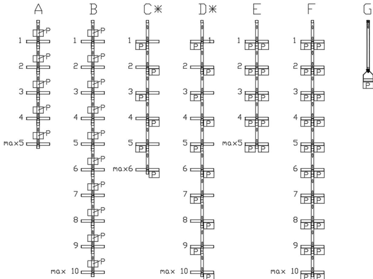
For the variants C\* and D\* the sum of loadings at the left and at the right side have to be equally. The number of frames has to be even.
